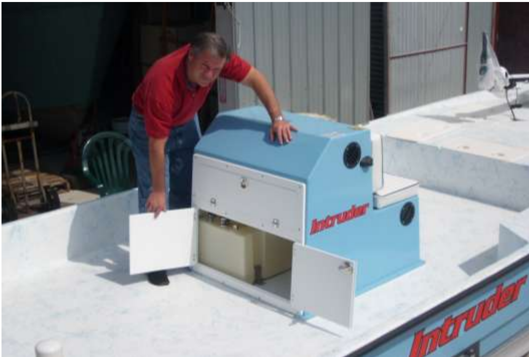
The bottom of the console stores a 27 gallon fuel tank. It is well vented with room for up to three batteries.
