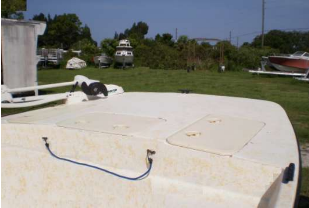
Forward platform has three compartments, one is converted to a bait well.
